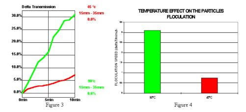
Calculation of the slope of the graph over 10 minutes allows the determination of the sediment formation speed as a function of the maximum temperature of the wort (Figure 4).
