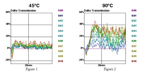
By plotting the variation of the transmission in the middle of both samples as a function of time (Figure 3) we get a quantitative comparison of the rate of flocculation.
