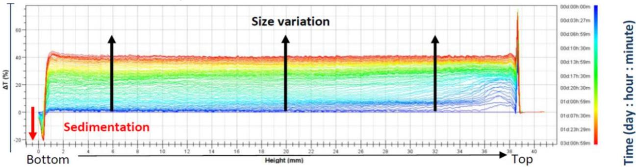
Figure 1: Transmission data of an IPA beer (sample A) - 3 days
