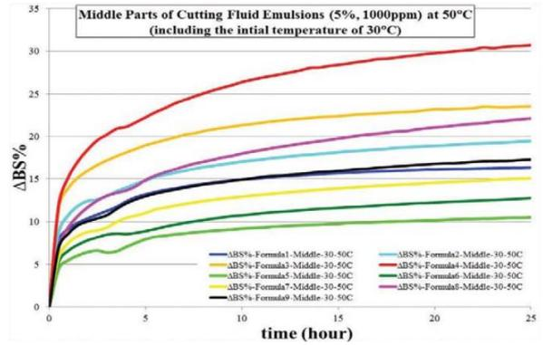
Figure 4: backscattering variation (%) in function of time for 9 sample tests
