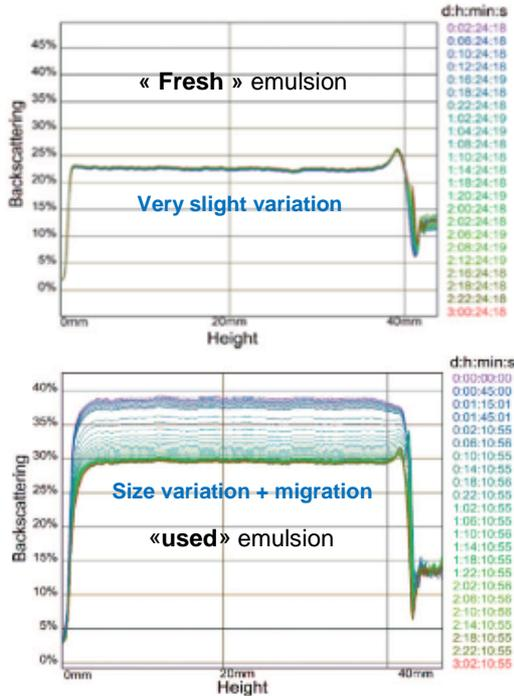
Figure 7: Backscattering signal obtained from wire drawing emulsion after (top) and before (bottom) their replacement.
