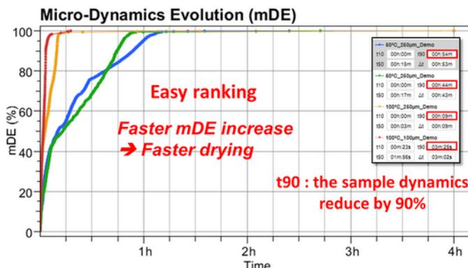
Figure 5: Micro-dynamics evolution function of time for cathode slurry at different temperature and different coating thickness
