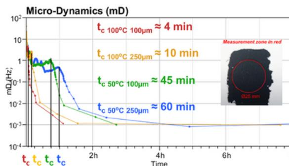
Figure 3: Micro-dynamics function of time for cathode slurry at different temperature and different coating thickness
