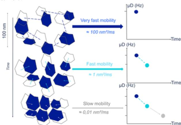
Figure 2 : Schematic representation of the mobility ( $\mu\text{D}$ ) evolution during typical drying/curing process versus time
