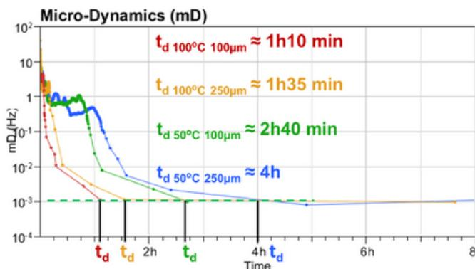
Figure 4: Curing time as a function of the curing temperature for an epoxy adhesive
