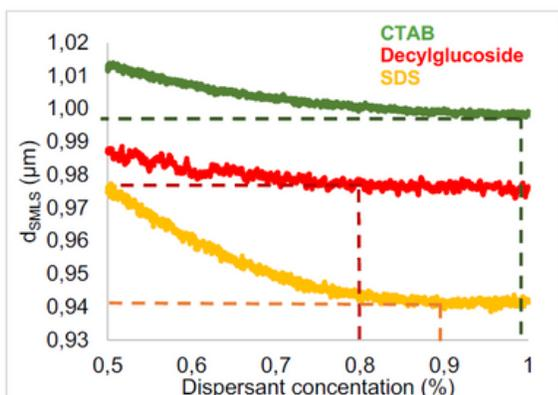
Figure 2. Zoom on particle size (µm) as a function of dispersant concentration (%wt) with optimal concentration.
