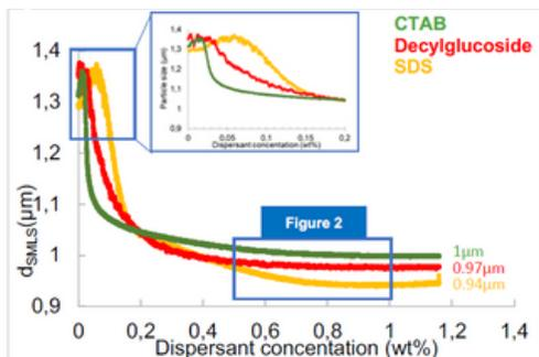
Figure 1. Particle size (µm) as a function of dispersant concentration %wt.
