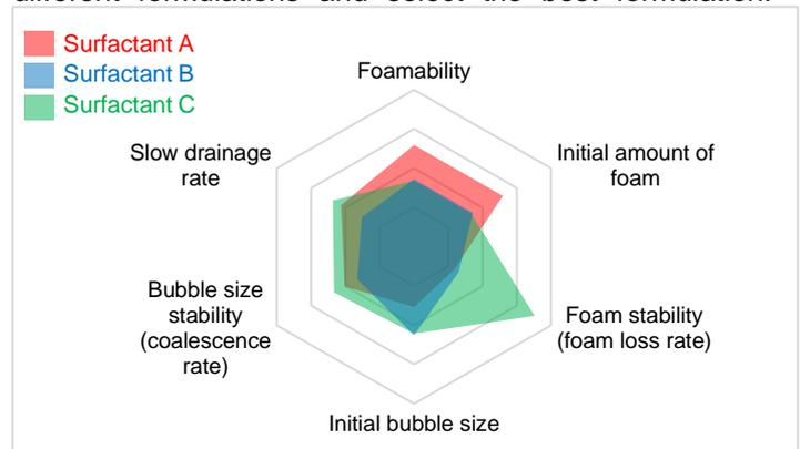
Surfactant B is surpassed in all the parameters by the surfactant A and C and can be considered as the least efficient foaming agent. For **foam generation**, **surfactant A** is the most appropriate foaming agent, it generates the most amount of foam, However the foam is not as **fine** and as **stable** as the foam generated by the **surfactant C**. So, for stability and for the finest foam, surfactant C is the surfactant of choice.
