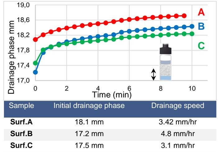
The foam generated by the surfactant C has the slowest drainage speed, which must be related to the bubble size (the smallest) and the stability of the foam.
