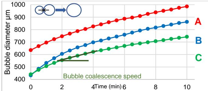
The bubble coalescence rate can easily be obtained by determining the slope of the kinetics:
