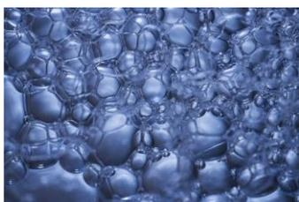
Foamability depends on surfactant nature, concentration, and the liquid phase viscosity. Foamability (related to the amount of foam generated) and foam stability are two separate properties to consider. There are three main process of foam destabilization:
