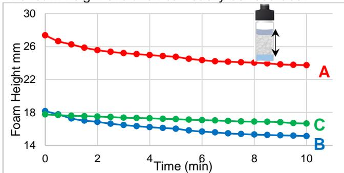
From the previous graph, the initial amount of foam can also be determined as well as the speed of foam loss (slope of the curve), thus the foams stability can be easily evaluated.
