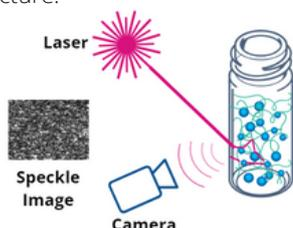
**Figure 1. Schematical representation of the measurement set-up.**
