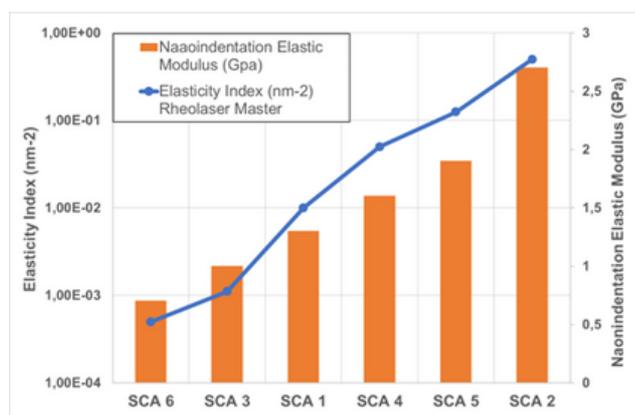
Figure 5. Comparison of measurements during gelation with Rheolaser Master and after 72 hours of drying with nanoindentation.
