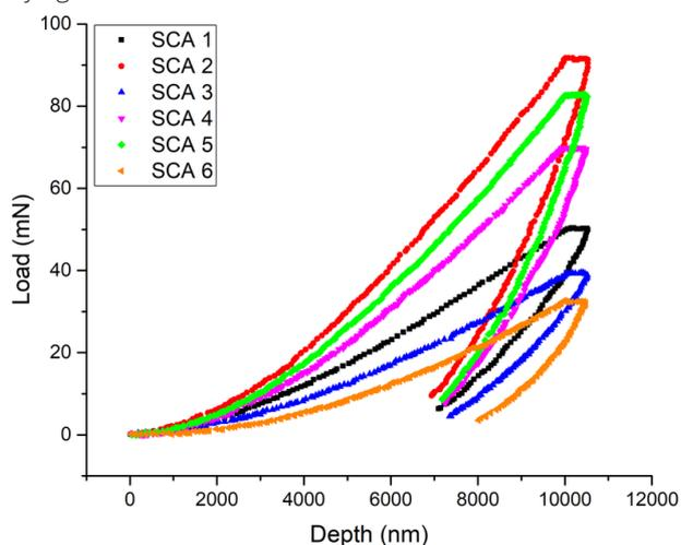
Figure 4. Mechanical tests using nanoindentation of 6 different ceramic inks after 72 hours.
